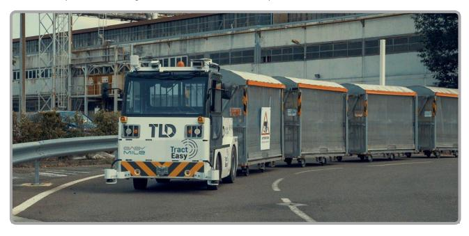
The TractEasy® has been co-developed with the French company EasyMile. Its mission is to move cargo in an autonomous manner, under the supervision of dedicated fleet manager software, from terminal to terminal, or terminal to aircraft.
